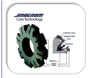
Magnom<sup>™</sup> core elements are comprised of an annular magnet and two innovatively formed steel plates. The steel plates direct the lubricant flow and magnetic flux through channels designed to bring all the ferrous contaminants in the lubricant within the range of the magnets.
